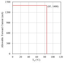
Figure 1.  $T_S$  vs Allowable Forward Current
